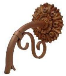
Penny Copper is an extra thick layer of copper plating over everything, the copper is left un-sealed, so it can verde naturally. This is useful because the backplate and the spout are different metals and the customer wanted an even natural Verde.
